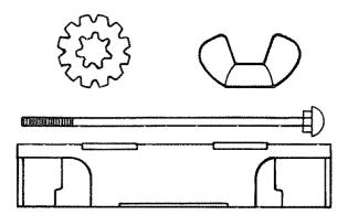
two Battery Bolts and one Terminal Guard found in Bag of Parts.
